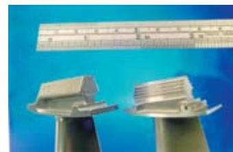
Turbine blade root forms.
