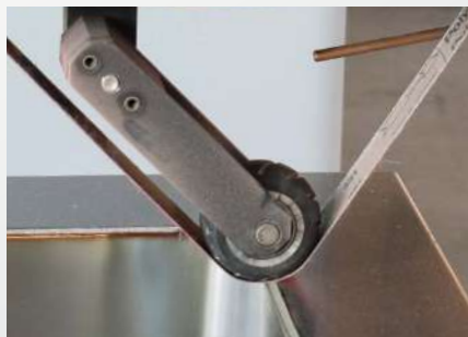
Grinding detail on welded seam with spraying nozzle.
