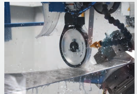
Grinding process – radial grinding Schleifprozess – radial schleifen
