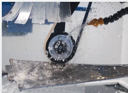
Grinding of smallest leading and trailing edges – longitudinal grinding
